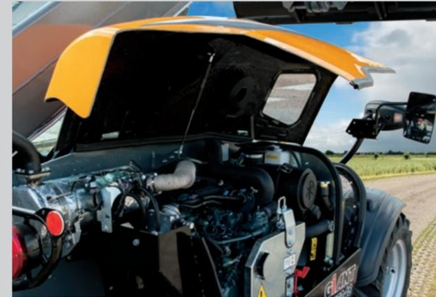
Performing maintenance to the GT5048 is no problem at all because the service points are easy to reach. Filters, hydraulic system and engine can be freely accessed via the easy-to-open bonnet, tilting cab or other service panels. This ensures that daily checks and maintenance can be carried out quickly and in a safe manner.
